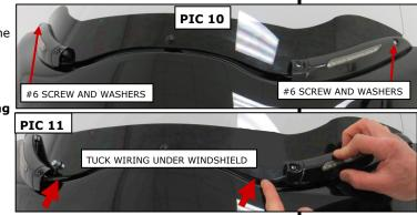
**STEP 22** Align the center trim piece over the side trim pieces and front standoffs; secure it with the two remaining #6 screws and washers. Alternately tighten all four screws.
