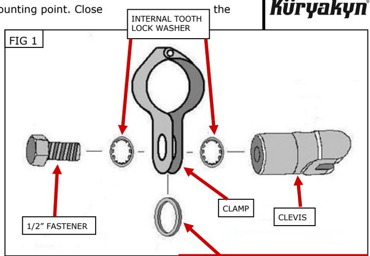
**WARNING** FOOTPEGS MUST BE INSTALLED SO THEY WILL FOLD UPWARD AND REARWARD IF HIT BY ANY OBJECT. FAILURE TO ADJUST THE FOOTPEGS TO OPERATE IN THIS MANNER COULD RESULT IN SERIOUS INJURY OR DEATH.
