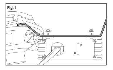
10. Using the (2) remaining 6-32 screws, washers, and lock-nuts, attach the amplifier to the already installed upper mounting bracket. (**Figure I**) Attach the lower mounting bracket to the lower right hand fairing mounting stud.
