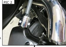
**STEP 6** Assemble the cover using the socket head cap screws removed in Step 4. Tighten securely.
