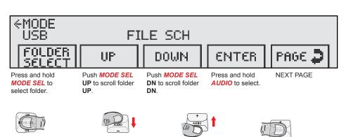
After pressing and holding <code>mode sel</code> to enter FOLDER SELECT mode, you must press and hold <code>audio</code> to confirm the FOLDER SELECT mode. After <code>audio</code> is pressed and held, you will see the first FOLDER on the USB. Push <code>audio</code> <code>UP</code>/DOWN until the desired folder is displayed. Press and hold <code>audio</code> to select the folder. Repeat steps to select a song in the folder.
